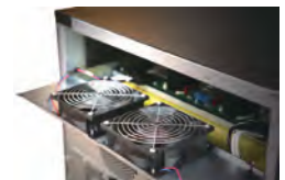
Redundant fan design enhances system reliability*
