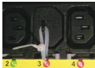
Cap secures in place with cable tie
