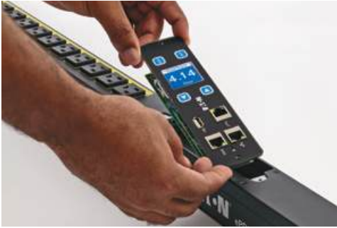
Module being removed without removing power to the ePDU
